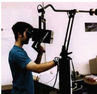
Fig. 2. A Binocular Omni-Orientation Monitor (BOOM)
