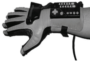
Fig. 5. An instrumented glove (Nintendo power glove)
